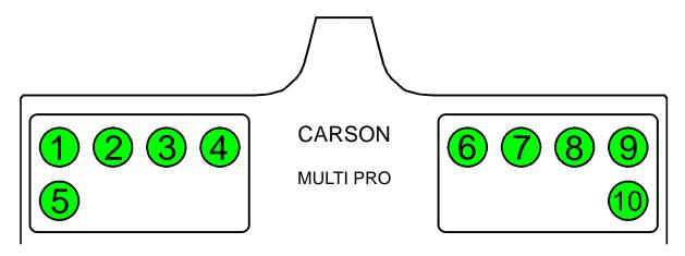
For the switches 1-10 two functions can be assigned in the Sound-Teacher or in the Drive-Teacher. One function for "switch up" and one function for "switch down". In total 20 additional functions can be switches with the MSC-10-C.
