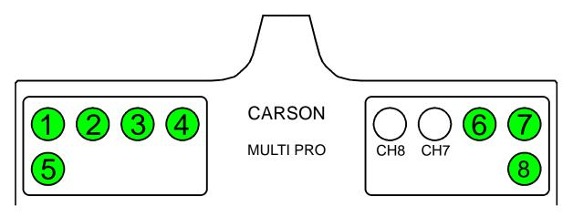
For the switches 1-8 two functions can be assigned in the Sound-Teacher or in the Drive-Teacher. One function for "switch up" and one function for "switch down". In total 16 additional functions can be switches with the MSC-8-C.
